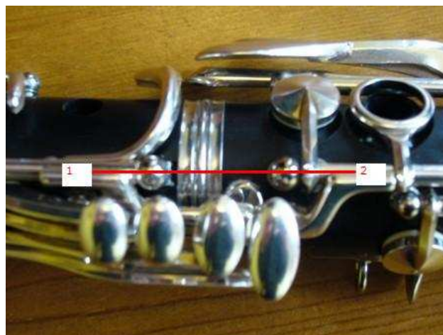
'Spines' of ring keys aligned.
